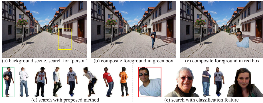
Fig. 1: Compositing-aware image search. Given a background image as a query, the task is to find foreground objects of a certain category that can be composited into the background at a specific location, as indicated by the rectangle.
